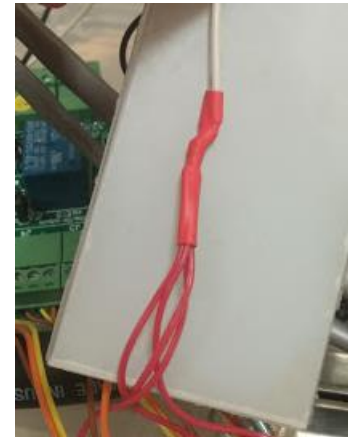
Figure 4.8 A proper junction between the stepper +5V inputs (red, bottom) and the +5V power supply output (white, top)
