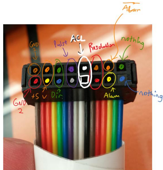
Figure 4.4 The female pin headers connecting to the breakout board. With reference to Figure 4.5, the ribbon cable would come off to the right when plugged in, and the GND pins would be topmost to match the male pins. Circled connections are wired together at the stepper driver pins.
