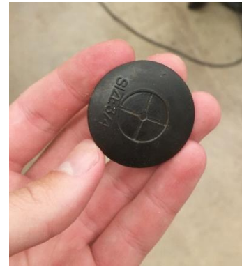
Figure 6.7 A grommet removed from its through hole. This one has not yet been cut open along its cross
